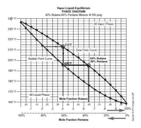
referred to as vapor-liquid-equilibrium (VLE) diagram or phase diagram.
